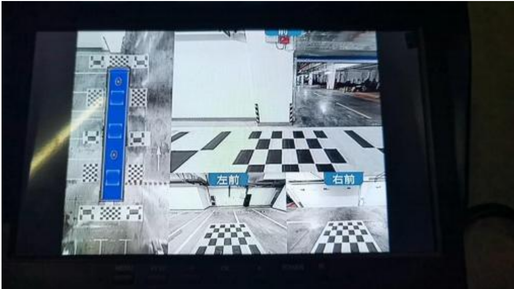
6-Way AVM (Around View Monitor) with BSD (Blind Spot Detection) for cranes.
